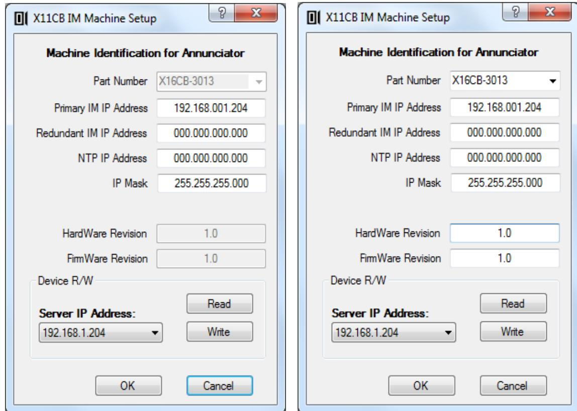
Figure 4-1 IM Machine Setup Security Level Differences
